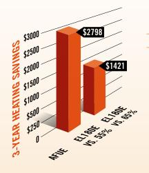
AFUE stands for "Annual Fuel Utilization Efficiency" and is a measure of a furnace's efficiency and performance. Like the miles-per-gallon rating on your car, the higher the AFUE rating, the lower your fuel costs.
